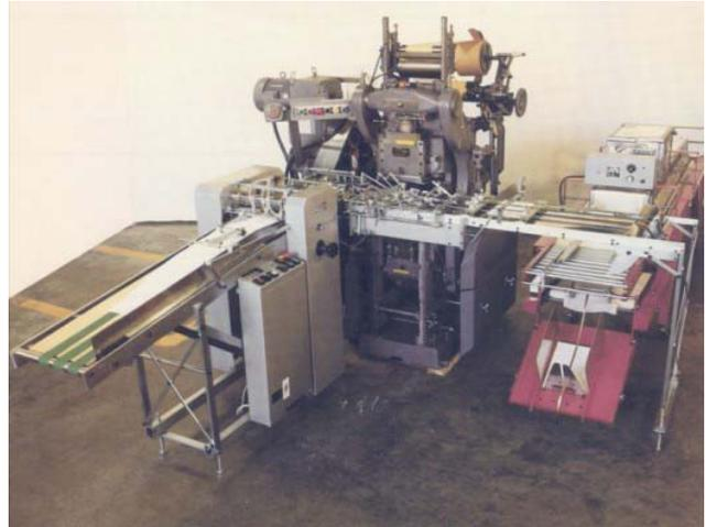
In 1946, Cronite began producing the 3 X 8 Press and by 1953, with the appearance of the Autofeed, emphasis was placed on increasing production capacity. Today's 3 X 8 ¾ Hi-Speed Die Stamping Press System (consisting of the Hi-Speed 3 X 8 ¾ Press, High Speed Autofeed, and Telestacker Drier) is the result of many years of engineering research devoted to modernizing the die stamping plant.
