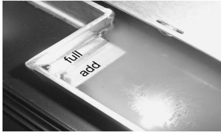
**Important:** During warm up, the coating roller gets heated up by the adhesive. It is very important that the level of the adhesive be above the “full” block (top block, located in the left side of the tray). If the adhesive is too low, the warm up will take longer and the roller will have trouble turning.
