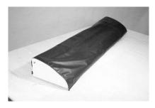
When you have finished coating, replace the black vinyl cover over the machine to reduce the thickening of the adhesive in the tray.
