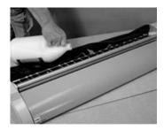
Pour the adhesive into the rear of the tray until the level reaches the upper label (full). There is also an 'add level' label.
