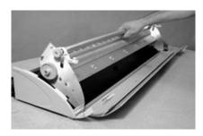
Holding the top roller, swivel the coating roller up and out of the tray.
