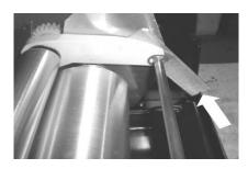
There are two support plates attached to the back arm which have a V groove in them. Hook the V groove to the steel base, to keep the assembly up.
