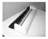
Place the Rollataq on a level surface and connect the machine to an approved outlet. Roll back or remove the black vinyl cover from the Velcro backing. The cover should be replaced when the machine is not being used as it keeps the adhesive fresh.
