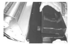
If you are not going to use the machine for an extended period of time you can cover the adhesive tray with the spare tray supplied. This will keep the adhesive fresh for up to two weeks. (note: stackable plastic trays in 24" model only, not 36")
