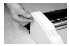
Remove the screws on both ends of the coater.
