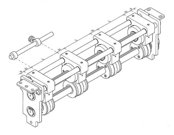
The Zip21A uses slitting and/or scoring blades mounted in a removable cassette to slit the paper as it passes through the machine.
