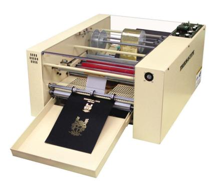
"Foil Fusing" or "Sublimation Foiling" is the method of bonding foil to a toner image printed by a copier machine or laser printer. Using Foil-Tech equipment, customers can now efficiently produce a wide range of high value products. Sheets up to 370mm (14½") wide by 610mm (24") long can be run through the machine.
