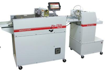
The new Zip-TS2L is a heavy duty, programmable cutter/slitter featuring a Windows XP touch screen control and *two* unique tooling stations that provide cross sheet scoring, perforating, die cutting, hole punching and blind embossing capabilities. The simple touch screen control allows a high degree of automation with fast set up, job program storage and retrieval. The programming is quick, simple and typically takes less than a minute to enter a new job.
