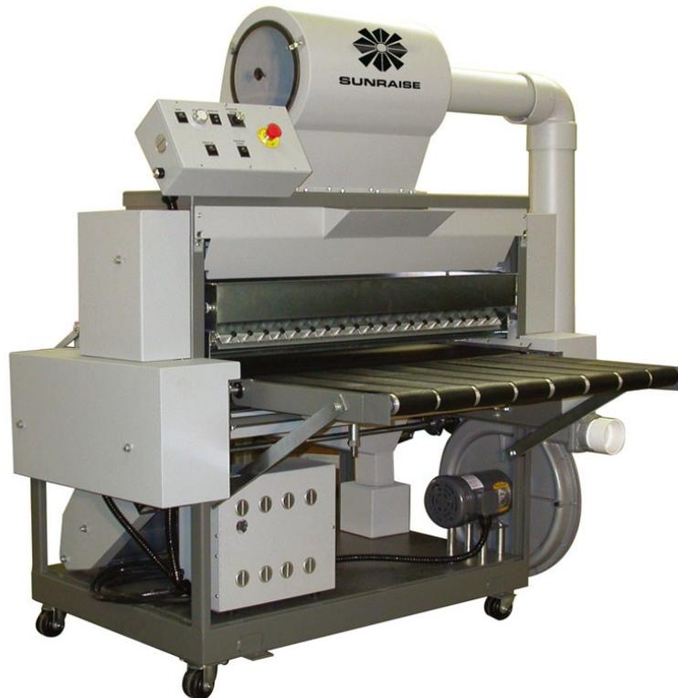
The PS Series, Powdering Section range of machines were specifically developed as stand alone, fully automated powdering section units for the application of adhesive powders used by the heat transfer industry.
