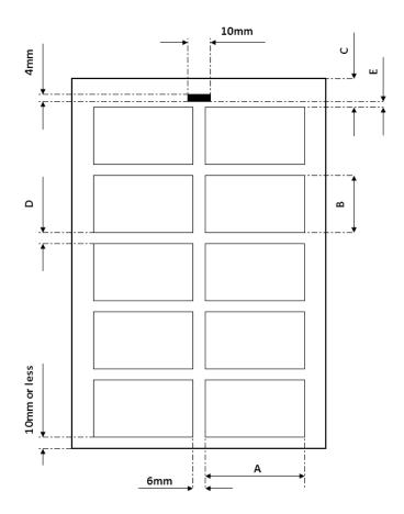
The diagram to the left shows the layout for the Zip10M.
